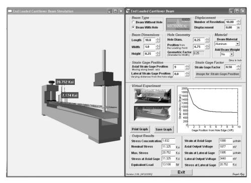
Fig. 4. Stand-alone cantilever beam simulation.
