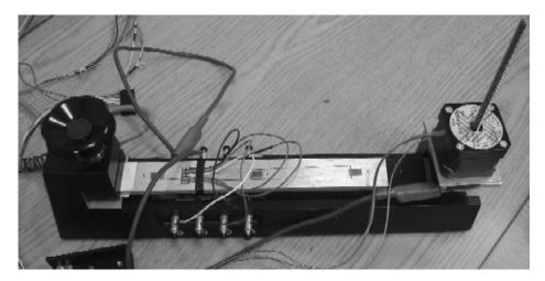
Fig. 1. Cantilever beam without stress raisers.
